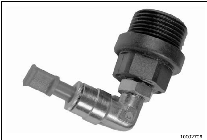
Fig. 18-5 Return-line connector, push-in type or screw type The return-line connection is designed to feed grease quantities that are not required back into the pump. It is installed instead of a closure plug (pump element).
