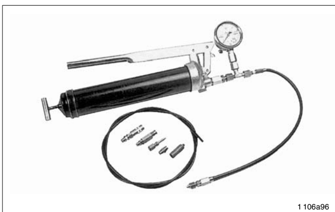
Fig. 24-5 Set for checking pressure and function: i.a. other hand-lever press 1142, pressure gage D63 0-600 bar and fitting Part no.: 604-36879-1
